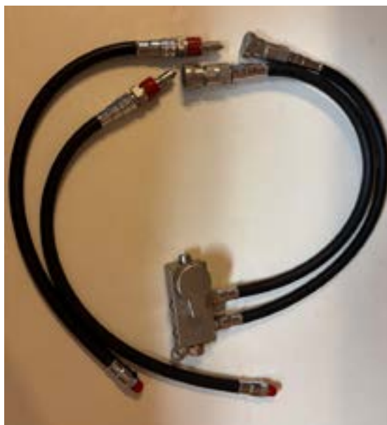
An example of a gas block with hoses. Courtesy of Michael A. Raymond.
