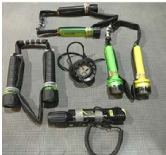
Head-mounted backup lights attached to repurposed bike inner tubes. One set is worn around the neck and another around the head when not wearing a helmet. Backup lights use non-rechargeable lithium batteries. Courtesy of Joe Kaffl.
