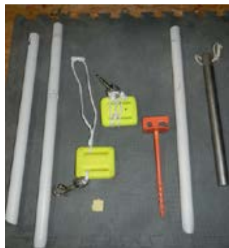
Sample of line belays L to R: Disler spikes; drop weight in stowed position with wrapped line with clip for attachment to D-ring; plastic screw for hard gravel, and 3-pound stainless weight to attach to side mounts. The 1"x1" tile is used to mark sensitive areas in dry passages. Courtesy of Joe Kaffl.
