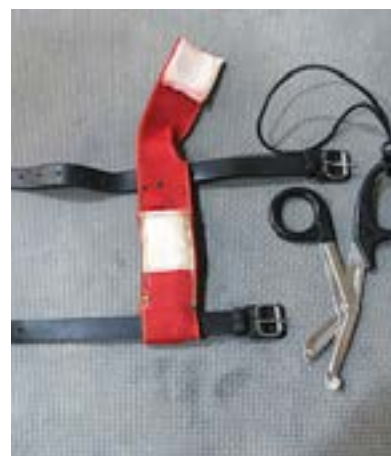
EMT scissors worn on wrist lanyard that allows them to dangle when doing line repairs and prevents inadvertent loss. Courtesy of Joe Kaffl.
